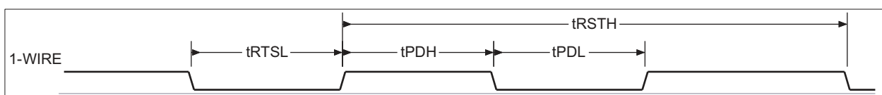
Figure 6-61. 1-Wire Break (Reset) Timing
