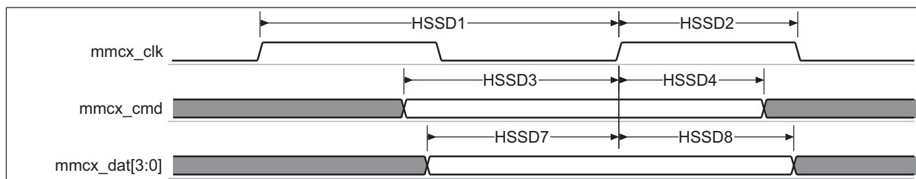
Figure 6-68. MMC/SD/SDIO High-Speed SD Mode Data/Command Receive
