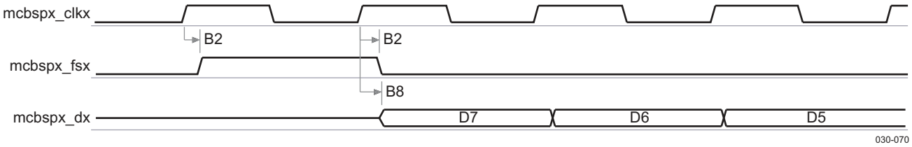
Figure 6-39. McBSP Rising Edge Transmit Timing in Master Mode
