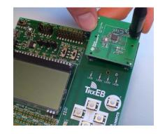
Insert a CC112xEM board into the TrxEB as shown above. Connect the antenna to the SMA connector on the EM.
