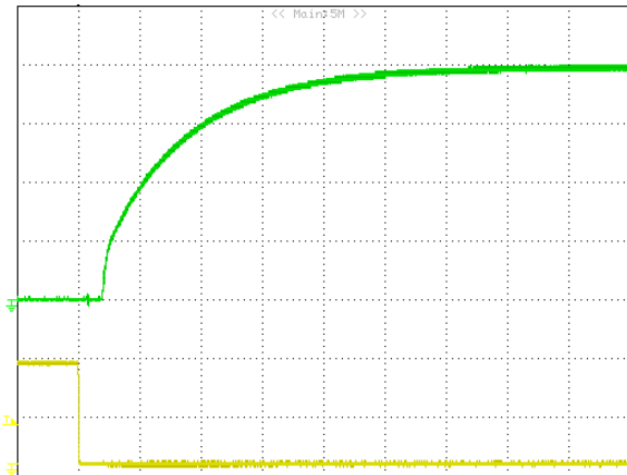
Figure 4: Turn-on transient at full rated load current (resistive load) (10 ms/div). Vin=48V. Top Trace: Vout, 3.0V/div; Bottom Trace: ON/OFF input, 3V/div
