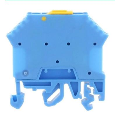
Disconnect terminal, Screw connection, Mounting type:Mounting rail TS 35/7.5 and TS 32, Rated cross-section: 2.5 mm², Width: 6 mm, Colour: Blue
