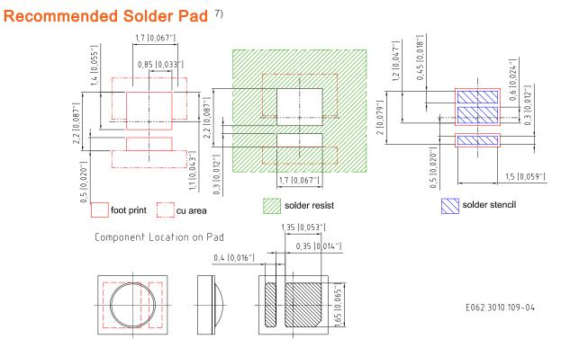
For superior solder joint connectivity results we recommend soldering under standard nitrogen atmosphere. Package not suitable for ultra sonic cleaning.
