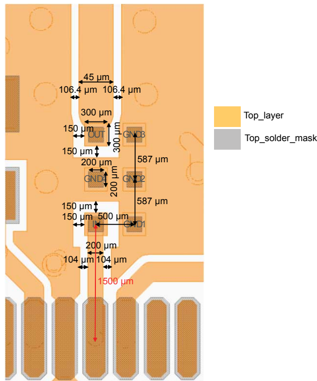
Figure 9. PCB land pattern recommendations
