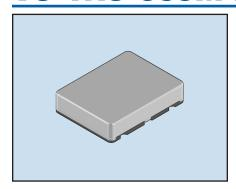
The VC-TXO-39SM is a VC (Voltage Controlled) TCXO (Temperature Compensated Crystal Oscillator) featuring very tight stability over a wide temperature range. The small SMD ceramic package measures  $11.4 \times 9.6 \times 2.3$  mm. The voltage control has a tuning range of  $\pm$  12 ppm typical. The low profile package is ideal for wireless communications applications.
