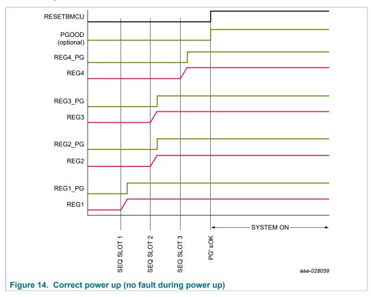
If any of the regulators are powered up before RESETBMCU is out of regulator, RESETBMCU is not de-asserted and the power up sequence is stopped for up to 2.0 ms. If the fault is cleared and all internal PG signals are asserted within the 2.0 ms timer, RESETBMCU is de-asserted and the power up sequence continues where it stopped as shown in Figure 15.
