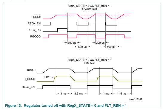
When the LDO2 is controlled by hardware using the LDO2EN pin and programmed to turn off upon an OV, UV or ILIM fault, the LDO2\_FLT\_REN bit still controls whether the regulator returns to its previous state or not regardless the state of the LDO2EN pin.
