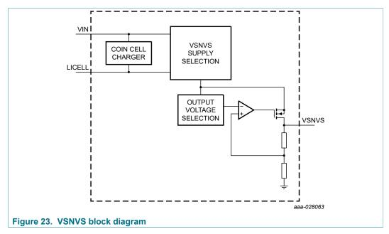
The VSNVS output keeps regulation through all states, including the system-on, off modes, power down sequence, watchdog reset, and fault transition as long as it has a valid input (VIN or LICELL), and the output has been configured by the OTP\_VSNVSVOLT[1:0] registers.
