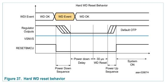
After a WD reset, the PMIC may enter the standby state depending on the status of STANDBY pin.
