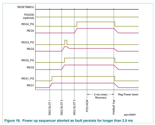
Supplies enabled after RESETBMCU are checked for OV, UV and ILIM faults after each of them is enabled. If an OV, UV or ILIM condition is present, the PF8121 starts a fault detection and protection mechanism as described in <a href="Section 14.7">Section 14.7</a> "Fault detection". At this point, the MCU should be able to read the interrupt and react upon a fault event as defined by the system.
