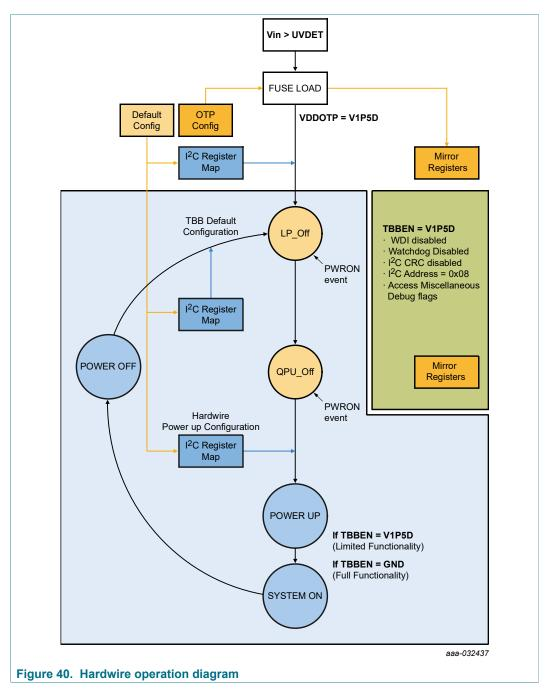
For simplicity, the default hardwire configuration in PF8121 is organized based on the OTP register map as shown in <u>Table 75</u>.
