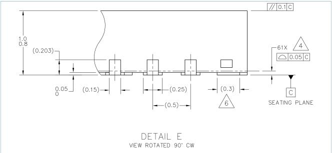
Figure 43. Package outline detail for E-type HVQFN56
