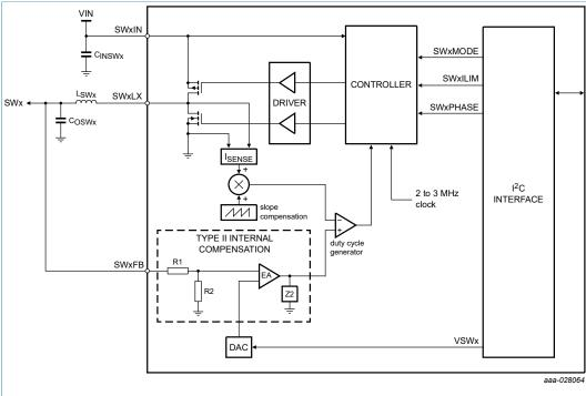
Figure 24. Buck regulator block diagram
