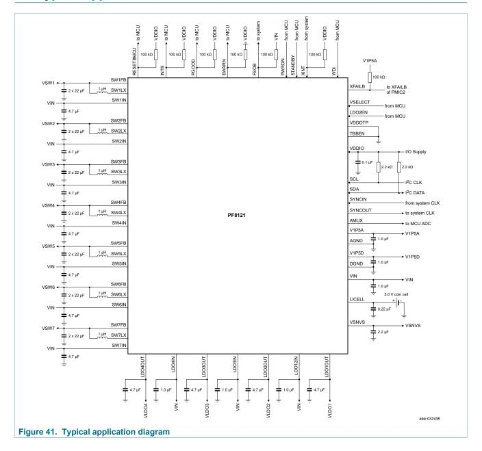
12-channel power management integrated circuit for high performance applications
