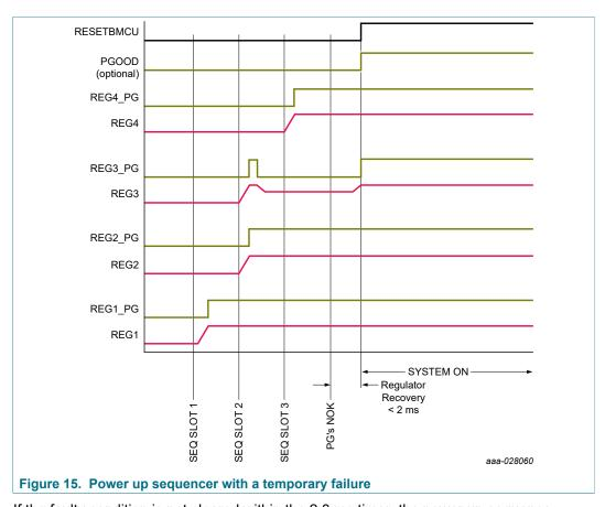
If the faulty condition is not cleared within the 2.0 ms timer, the power up sequence is aborted and the PF8121 turn off all voltage regulators enabled so far as shown in Figure 16.
