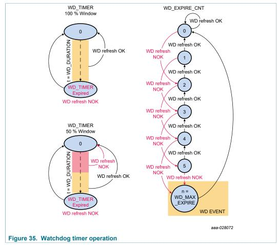
The watchdog function can be enabled or disabled by writing the WD\_EN bit on the  $I^2C$  register map. When the  $I^2C$  secure write must be performed to change the WD\_EN bit.
