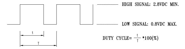
THE FREQUENCY FOR CONTROL SIGNAL OF THE FAN SHALL BE ABLE TO ACCEPT A 10KHZ.
