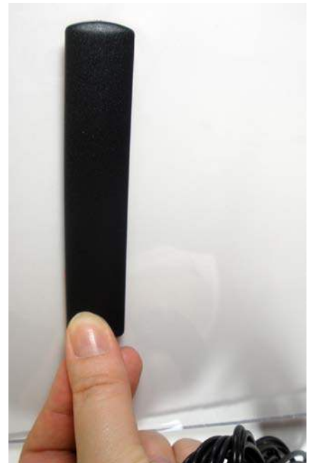
Figure 20. Adhesive Mount Antenna – Step 3. Mount the Antenna
