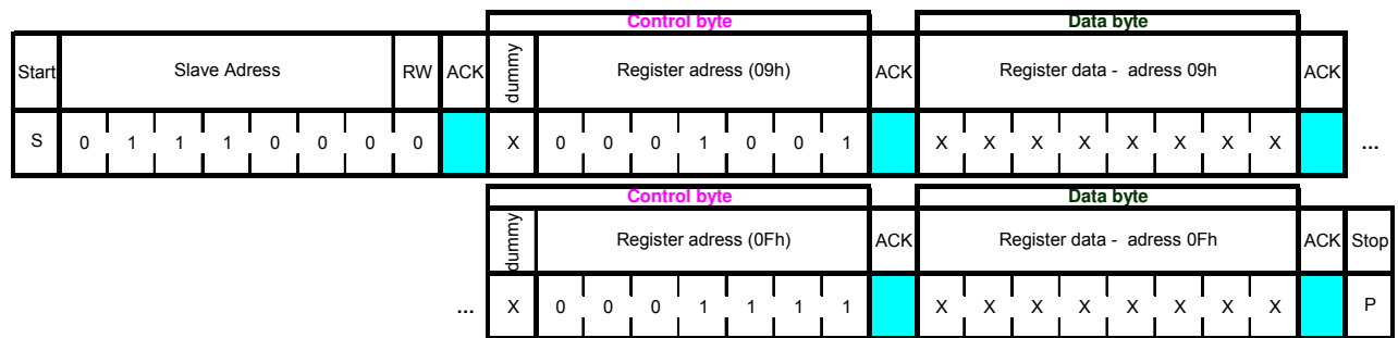
Figure 15: I 2 C multiple write protocol
