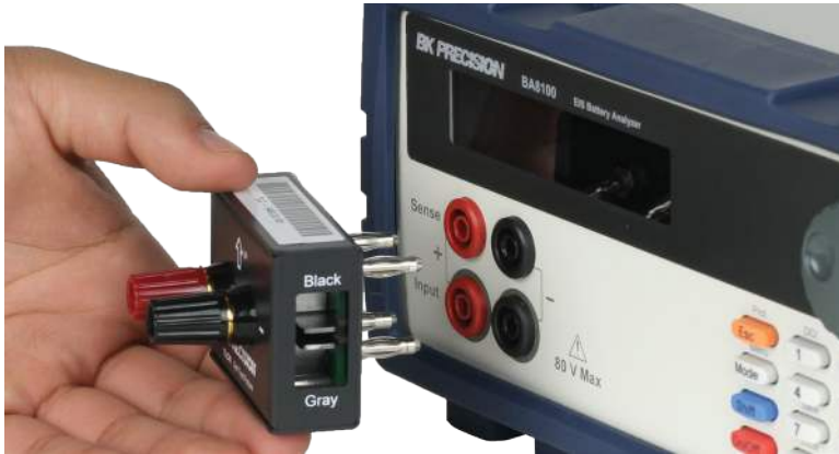
TLC81 plugged-in to the front panel
