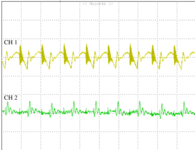
Figure 9: 3.3V and 5.0V output ripple/noise (2uS/div): CH1: Vo, 3.3V (50mV/div). CH2: Vo, 5.0V (50mV/div).
