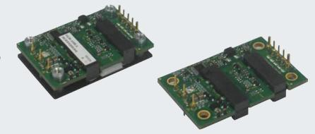
Advanced Energy's Artesyn AVQ100-24S05 is a single output DC-DC converter with standard quarter-brick outline and pin configuration. It delivers up to 20A output current with 5V output voltage. Above 93% ultra-high efficiency and excellent thermal performance makes it an ideal choice in telecom and datacom application.
