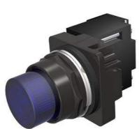
30mm BlackMax, Epoxy Coated Corrosion Resistant Complete Metal Unit Illuminated Indicator Light Transformer type, 120V AC LED Lamp, BA9s Plastic Lens, Blue UL Listed, CSA Certified NEMA 1,3,3R,4,4X,12,13 & Automotive Standards
