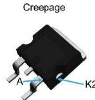
Figure 22. Creepage without top coating
