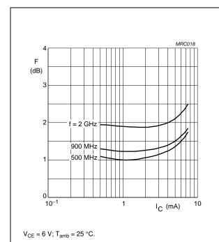
Fig.10 Minimum noise figure as a function of collector current.
