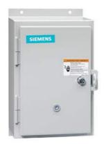
Non-reversing motor starter, Size 0, Three phase full voltage, Solid-state overload relay, OLRelay amp range 0.75-3.4a, 550/575 600 50/60HZ coil, Non-combination type, Enclosure type 12, Dust/drip proof for indoors, Extra-wide enclosure
