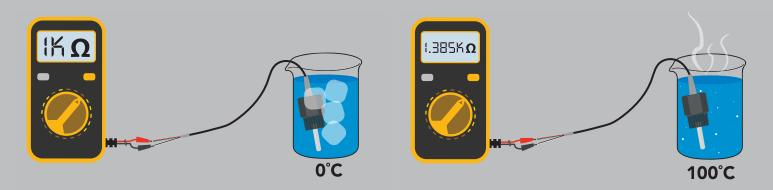
To convert the resistance of the probe to temperature, use the following simplified equation:
