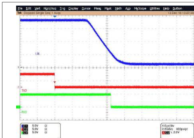
Figure 10-11. Recessive to Dominant Propagation Delay
