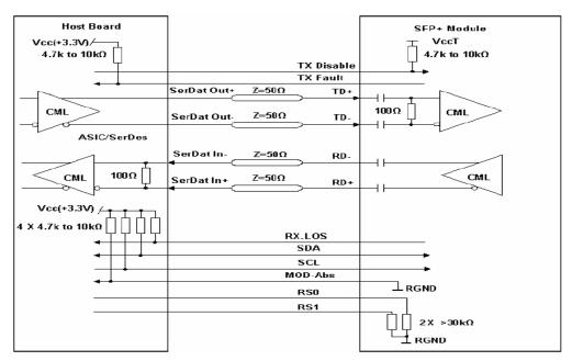
**Recommended High-speed Interface Circuit**
