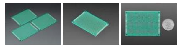
Here's a handy 3-pack of 5cm x 7cm Proto-board PCBs in green. Both sides have a green silkscreen with some row/column markings. Note that these *don't* have any traces between the PCB holes, <u>you would normally bend over a thru-hole lead to create connections</u>. They're also good for just plain mechanical work because they are made of strong FR4.
