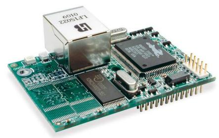
integrated features and a C-friendly instruction set designed for use with the Dynamic C® development system. The RabbitCore mounts on a user-designed motherboard and acts as the controlling microprocessor for the user's system. Small in size but packed with powerful features, these core modules give designers a complete package for control and communication.
