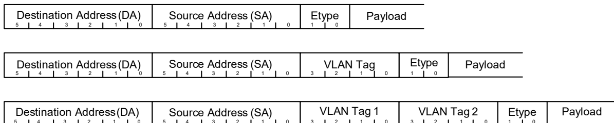
Figure 44 • Type II Ethernet Basic Frame Format
