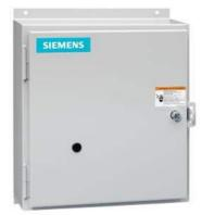
Non-reversing NEMA contactor, Size 2, Three phase full voltage, Contactor amp rating 45A, 3 wire (NO aux included), 190-220/220-240V 50/60Hz coil, Noncombination type, Enclosure NEMA type 12, Dust/drip proof for indoors, Extra-wide enclosure
