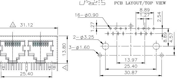
\* UNLESS OTHERWISE SPECIFIED TOLERANCES ON DECIMAL IS: ANGLE X.\*  $\pm$  3\* X.X\*  $\pm$  1\* UNIT: MM X.  $\pm$  0.30 X.X  $\pm$  0.25 X.XX  $\pm$  0.20 X.XXX  $\pm$  0.15
