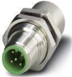
Sensor/actuator control cabinet feed-through, male to female, 5-pos., M12, shielded, A-coded, bipolar/screw mounting with M16 thread
