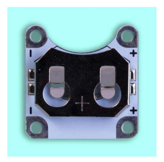
A lightweight, sewable battery board that's great for paper and fabric engineering projects. Works with CR2032 coin cell batteries.
