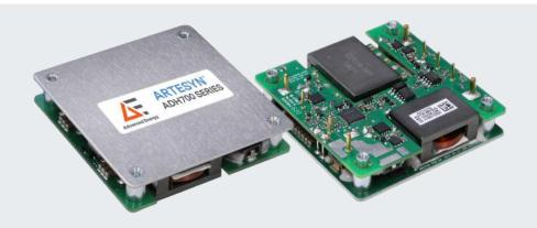
Advanced Energy's Artesyn ADH700 series half-brick isolated DC-DC converter provides a single regulated low noise output. ADH700-48S28 with 28V/25A output. It has a telecom input range of 36 to 65Vdc and is designed primarily for use with standard 48 V telecommunications equipment supplies. The converter's main application area is in low power and remote radio head (RRH) telecommunications applications.
