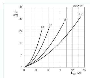
$$\begin{split} I_{F(AV)} &= I_{F(RMS)} \times \sqrt{\delta} \\ V_o &= 0.997 \text{ V; } R_s = 0.1192 \text{ } \Omega \end{split}$$
