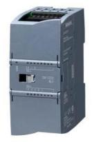
SIPLUS S7-1200 SM 1222 8DQ RLY based on 6ES7222-1HF32-0XB0 with conformal coating, -40...+70  $^{\circ}$ C, start up -25  $^{\circ}$ C, digital output 8 DQ, relay 2 A
