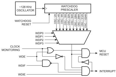
The WDT gives an interrupt or a system reset when the counter reaches a given time-out value. In normal operation mode, it is required that the system uses the WDR - Watchdog Timer Reset - instruction to restart the counter before the time-out value is reached. If the system doesn't restart the counter, an interrupt or system reset will be issued.
