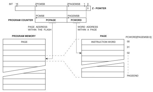
Figure 20-1. Addressing the Flash During SPM <sup>(1)</sup>
