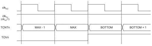
Figure 10-9 shows the same timing data, but with the prescaler enabled.
