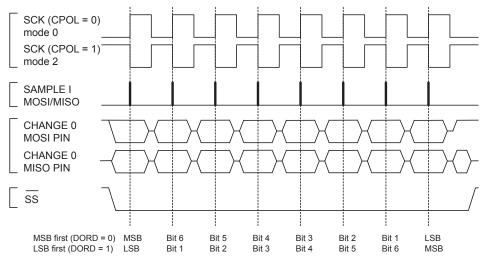
Figure 13-4. SPI Transfer Format with CPHA = 1
