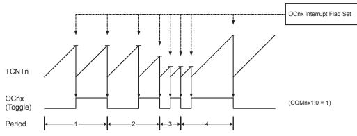
Figure 10-5. CTC Mode, Timing Diagram
