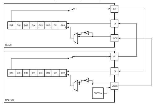
Figure 14-2. Three-wire Mode Operation, Simplified Diagram
