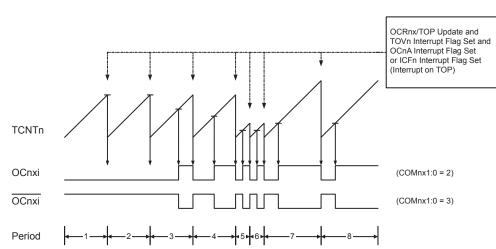
Figure 12-8. Fast PWM Mode, Timing Diagram
