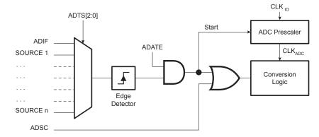
Using the ADC Interrupt Flag as a trigger source makes the ADC start a new conversion as soon as the ongoing conversion has finished. The ADC then operates in Free Running mode, constantly sampling and updating the ADC Data Register. The first conversion must be started by writing a logical one to the ADSC bit in ADCSRA register. In this mode the ADC will perform successive conversions independently of whether the ADC Interrupt Flag, ADIF is cleared or not.
