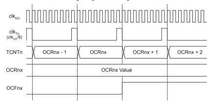
Figure 12-12. Timer/Counter Timing Diagram, Setting of OCF1A/B, with Prescaler (f<sub>clk\_I/O</sub>/8)
