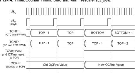
Figure 12-14. Timer/Counter Timing Diagram, with Prescaler (f<sub>clk I/O</sub>/8)
