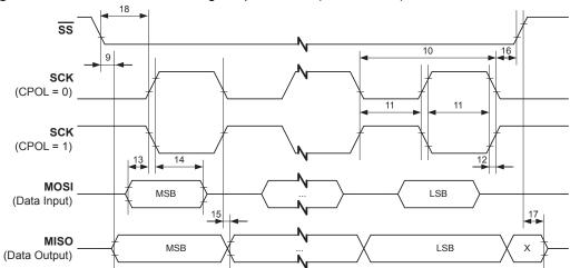
Figure 22-7. SPI Interface Timing Requirements (Slave Mode)
