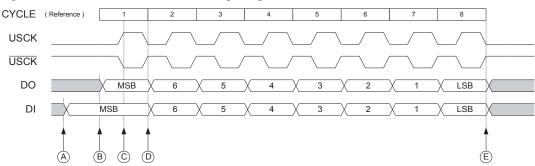
Figure 14-3. Three-wire Mode, Timing Diagram
