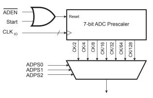
By default, the successive approximation circuitry requires an input clock frequency between 50 kHz and 200 kHz to get maximum resolution. If a lower resolution than 10 bits is needed, the input clock frequency to the ADC can be higher than 200 kHz to get a higher sample rate.
