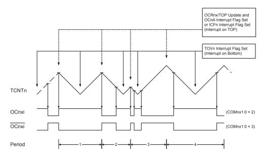
Figure 12-9. Phase Correct PWM Mode, Timing Diagram
