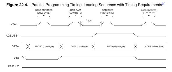
Note: 1. The timing requirements shown in Figure 22-3 (i.e., t<sub>DVXH</sub>, t<sub>XHXL</sub>, and t<sub>XLDX</sub>) also apply to loading operation.
