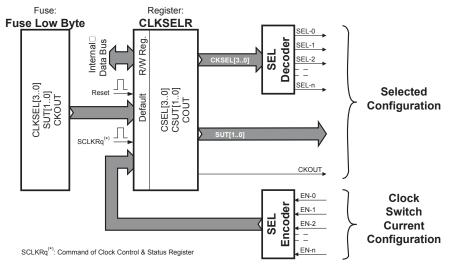
Figure 4-5. Fuses substitution and Clock Source Selection
