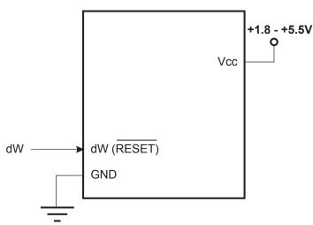
Figure 19-1 shows the schematic of a target MCU, with debugWIRE enabled, and the emulator connector. The system clock is not affected by debugWIRE and will always be the clock source selected by the CKSEL Fuses.
