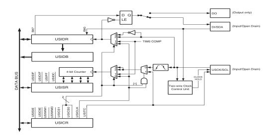
The 8-bit USI Data Register is directly accessible via the data bus and contains the incoming and outgoing data. The register has no buffering so the data must be read as quickly as possible to ensure that no data is lost. The USI Data Register is a serial shift register and the most significant bit that is the output of the serial shift register is connected to one of two output pins depending of the wire mode configuration.
