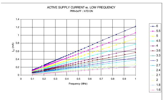
Figure 24-1. Active Supply Current vs. Low Frequency (0.1 - 1.0 MHz)
