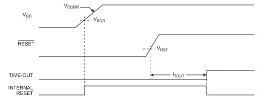
Figure 6-3. MCU Start-up, RESET Extended Externally
