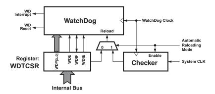
The 'Enable Watchdog in Automatic Reload Mode' command has priority over the standard watchdog enabling. In this mode, only the reset function of the watchdog is enabled (no more watchdog interrupt). The WDP3..0 bits of the WDTCSR register always determine the watchdog timer prescaling.
