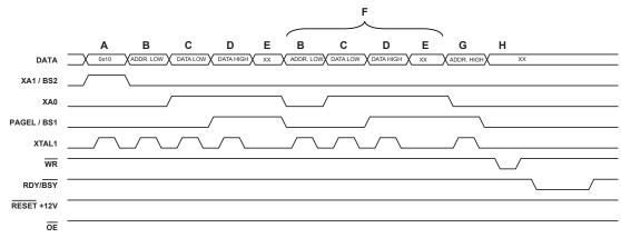
**Figure 21-3.** Programming the Flash Waveforms <sup>(1)</sup>
