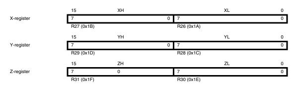
In the different addressing modes these address registers have functions as fixed displacement, automatic increment, and automatic decrement (see the instruction set reference for details).
