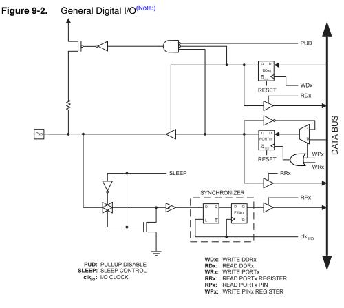
Note: WRx, WPx, WDx, RRx, RPx, and RDx are common to all pins within the same port. clk<sub>I/O</sub>, SLEEP, and PUD are common to all ports.
