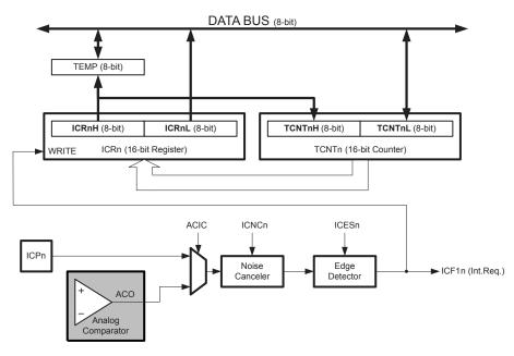
Figure 12-3. Input Capture Unit Block Diagram
