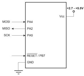
Note: If the device is clocked by the internal Oscillator, it is no need to connect a clock source to the XTAL1 pin
