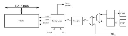
Figure 10-2. Counter Unit Block Diagram
