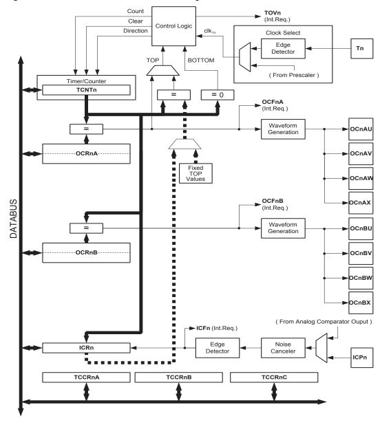
Figure 12-1. 16-bit Timer/Counter1 Block Diagram<sup>(1)</sup>
