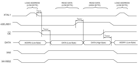
Note: The timing requirements shown in Figure 22-3 (i.e., t<sub>DVXH</sub>, t<sub>XHXL</sub>, and t<sub>XLDX</sub>) also apply to reading operation.
