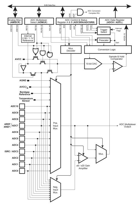
Figure 17-1. Analog to Digital Converter Block Schematic
