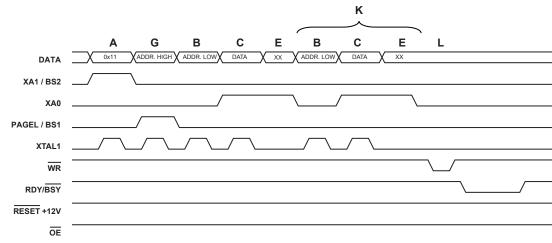
Figure 21-4. Programming the EEPROM Waveforms
