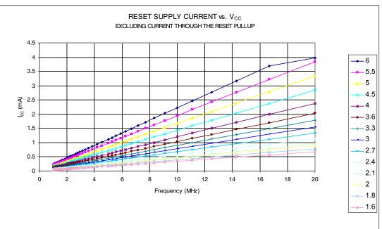
Figure 24-21. Reset Supply Current vs. Vcc, Frequencies ≥ 1 MHz (Excluding Current Through the Reset Pull-up)
