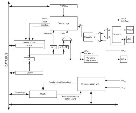
Figure 10-1. 8-bit Timer/Counter0 Block Diagram
