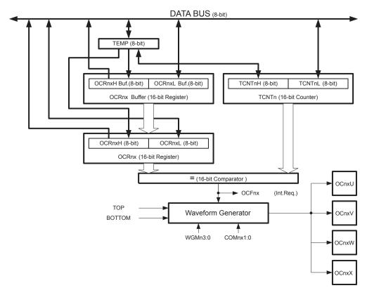
Figure 12-4. Output Compare Unit, Block Diagram
