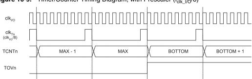
Figure 10-9. Timer/Counter Timing Diagram, with Prescaler ( $f_{clk \ I/O}$ /8)
