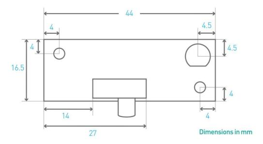
The 2 mounting holes are 3.3mm diameter.
