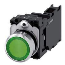
Illuminated pushbutton, 22 mm, round, metal, shiny, green, pushbutton, flat, momentary contact type, with holder, 1 NO+1 NC, LED module with integrated LED 230 V AC, Spring-type terminal
