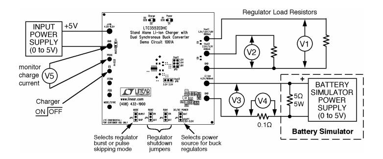
Figure 1. Demonstration Circuit Test Setup
