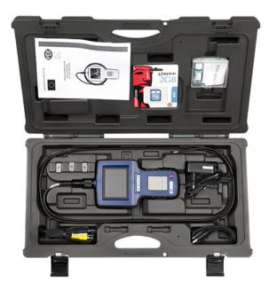
PCE-VE 320N is an industrial borescope, inspection camera or industrial endoscope for the non-destructive inspection (NDI) of engines, machines and more. This industrial borescope is an ideal tool for diagnosing issues in hard-to-reach places. The waterproof camera head features 4 LED lights with automatic illumination. In addition, digital image magnification or zoom of up to 2 times is available.
