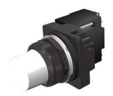
30mm BlackMax, Epoxy Coated Corrosion Resistant Complete Metal Unit Illuminated Indicator Light Full Voltage type, 24V AC/DC Incandescent Lamp, BA9s Glass Lens, White UL Listed, CSA Certified NEMA 1,3,3R,4,4X,12,13 & Automotive Standards
