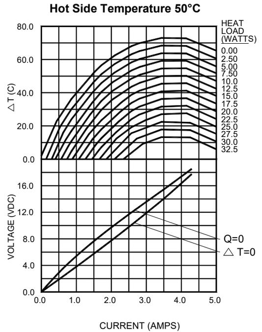
For performance information in a vacuum or with hot side temperatures other than 27°C or 50°C, contact one of our Applications Engineers at 877-627-5691.
