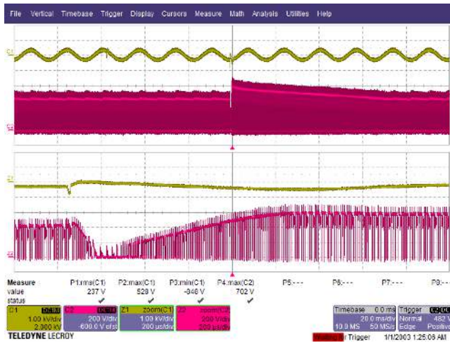
Figure 139 – DM Surge. V_{DS(MAX)} = 702 \text{ V} .
