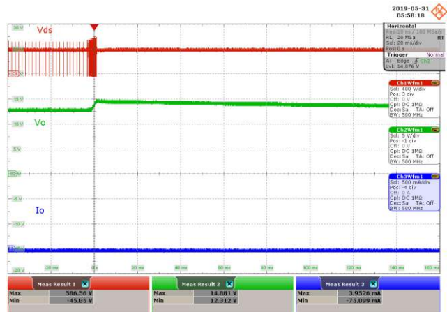
Figure 86 – 265 VAC 50 Hz, No-Load. CH1: V_{DS} , 400 V / div., 20 ms / div. CH2: V_{OUT} , 5 V / div., 20 ms / div. CH3: I_{OUT} , 500 mA / div., 20 ms / div. V_{OUT(MAX)} = 14.881 V.
