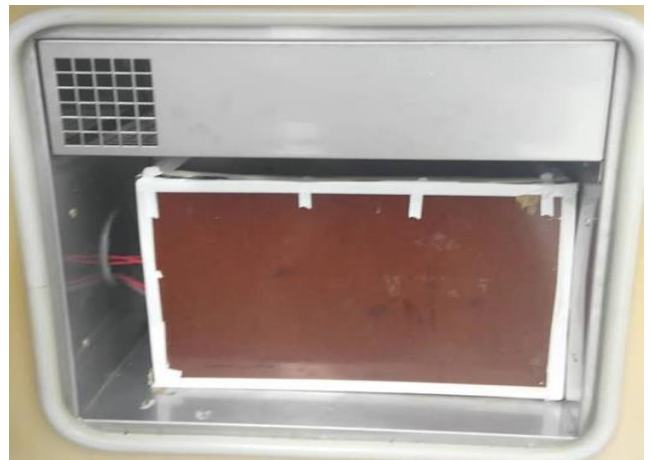
Figure 127 – Thermal Performance Set-up Using Thermal Chamber.
