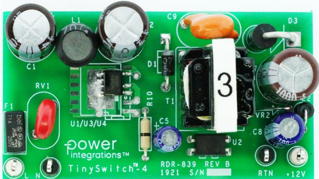
Figure 1 – Populated Circuit Board, Top View.
