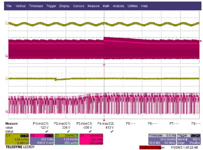
Figure 140 – CM Surge. V_{DS(MAX)} = 613 \text{ V}
