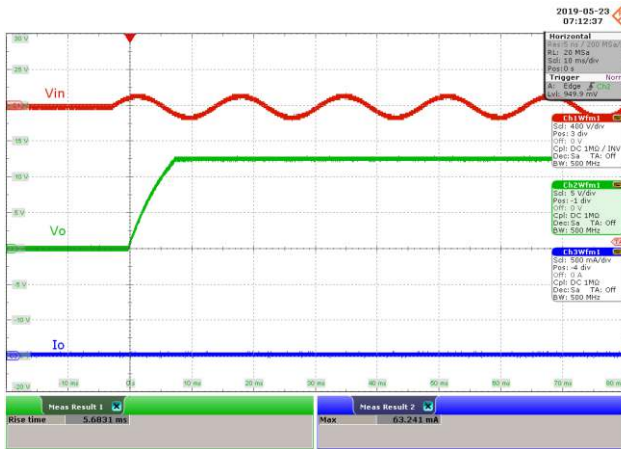
Figure 35 – 85 VAC 60 Hz. CH1: V_{IN} , 400 V / div., 10 ms / div. CH2: V_{OUT} , 5 V / div., 10 ms / div. CH3: I_{OUT} , 500 mA / div., 10 ms / div. Rise Time = 5.6831 ms.
