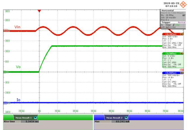
Figure 36 – 115 VAC 60 Hz. CH1: V_{IN} , 400 V / div., 10 ms / div. CH2: V_{OUT} , 5 V / div., 10 ms / div. CH3: I_{OUT} , 500 mA / div., 10 ms / div. Rise Time = 5.3454 ms.
