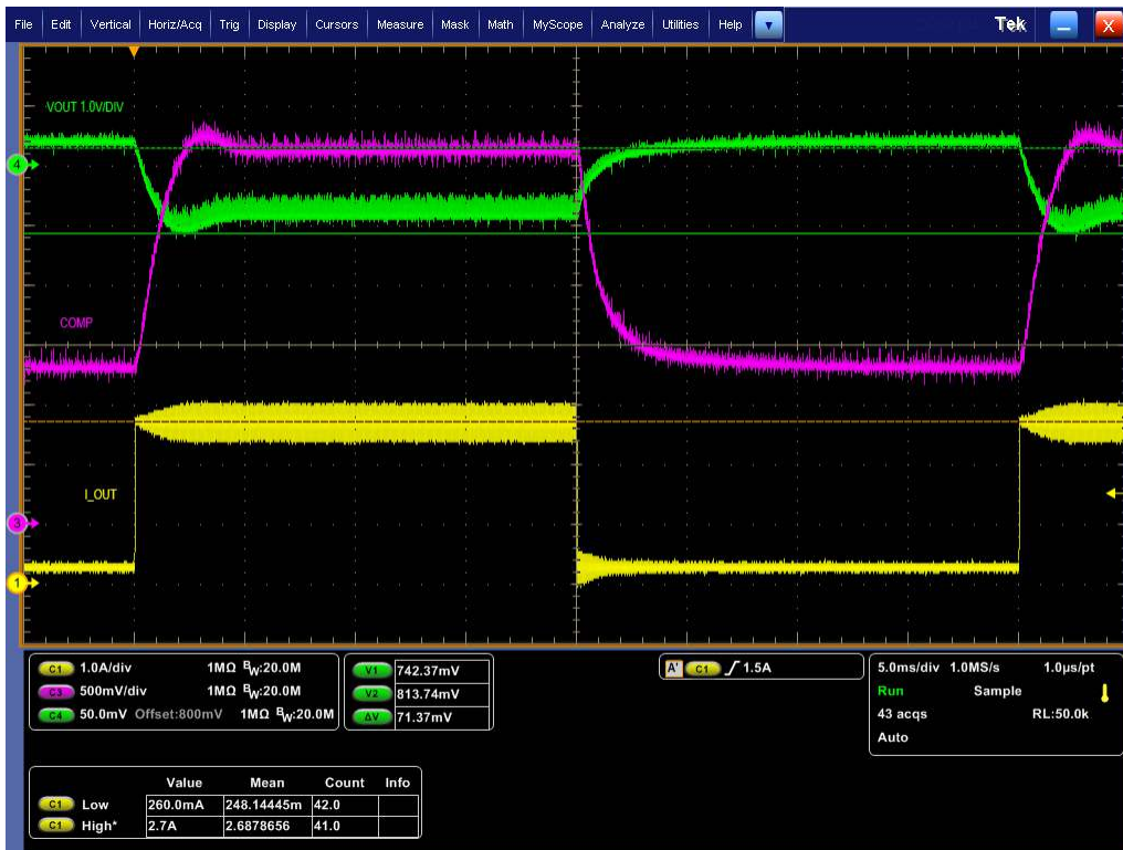
Figure 5-26. Transient Response: VIN = 800 V, Load = 0.25 A to 2.7 A at 25 Hz, 50% duty
