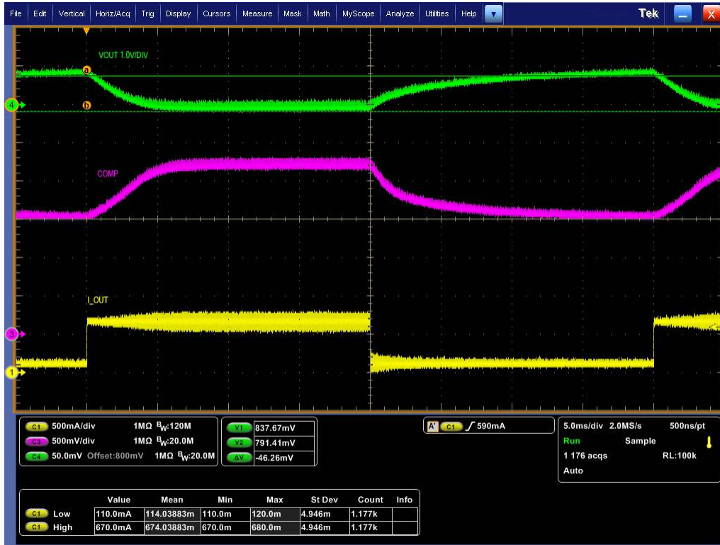
Figure 5-23. Transient Response: VIN = 50 V, Load = 100 mA to 650 mA at 25 Hz, 50% duty
