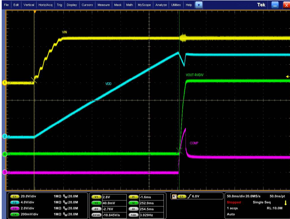
Figure 5-7. Start-Up 1: VIN = 50 V, Load = 0.25 A
