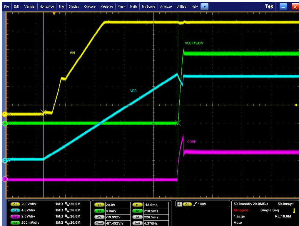
Figure 5-10. Start-Up 4: VIN = 1000 V, Load = 2.7 A
