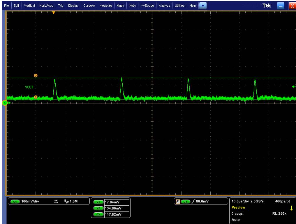
Figure 5-15. Output Voltage Ripple: VIN = 50 V, Load = 0.25 A
