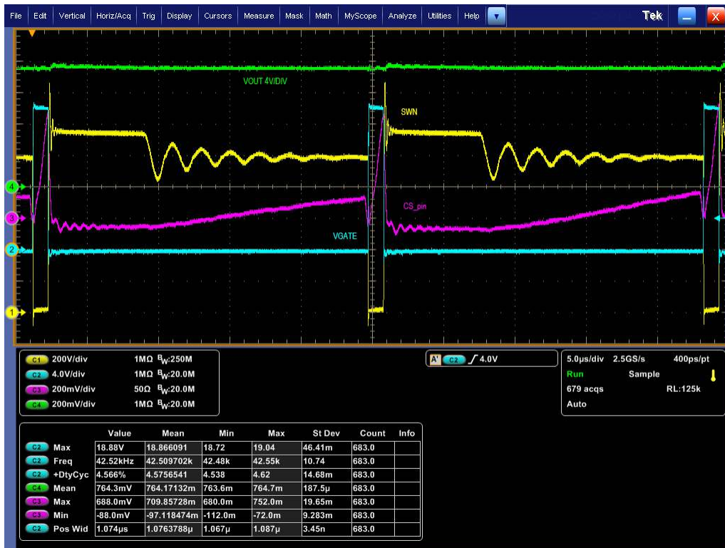
Figure 5-22. Steady State: VIN = 1000 V, Load = 2.7 A
