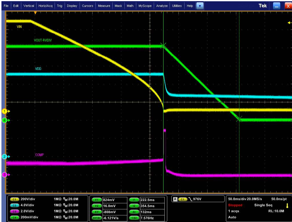
Figure 5-13. Shutdown, VIN Removal: VIN = 1000 V, Load = 0.25 A
