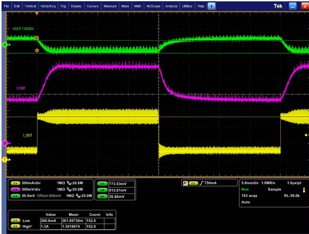
Figure 5-25. Transient Response: VIN = 800 V, Load = 0.25 A to 1.3 A at 25 Hz, 50% duty
