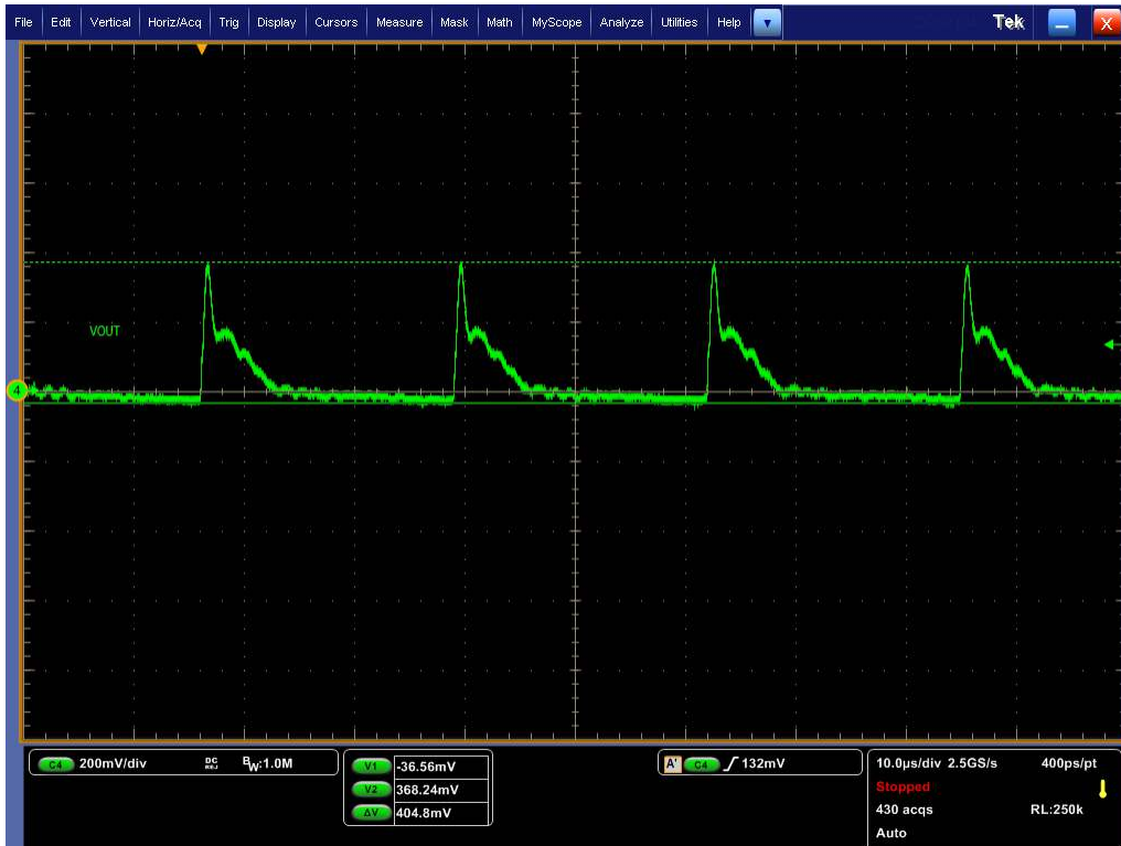
Figure 5-18. Output Voltage Ripple: VIN = 1000 V, Load = 2.7 A
