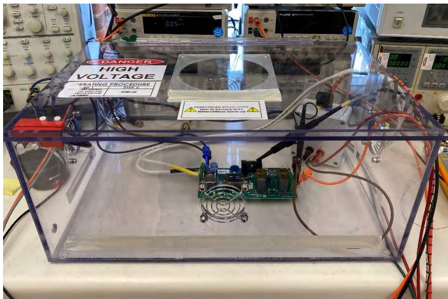
Figure 5-35. UCC28C56H EVM in plexiglass enclosure for HV safety. Virtually no airflow.
