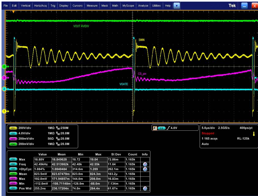
Figure 5-21. Steady State: VIN = 1000 V, Load = 0.25 A
