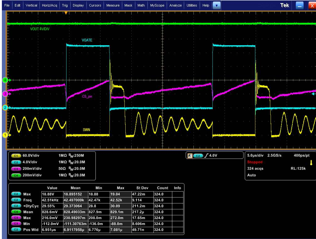
Figure 5-19. Steady State: VIN = 50 V, Load = 0.25 A
