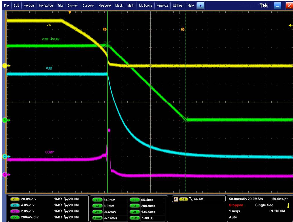
Figure 5-11. Shutdown, VIN Removal: VIN = 50 V, Load = 0.25 A
