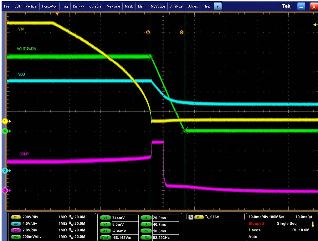
Figure 5-14. Shutdown, VIN Removal: VIN = 1000 V, Load = 2.7 A
