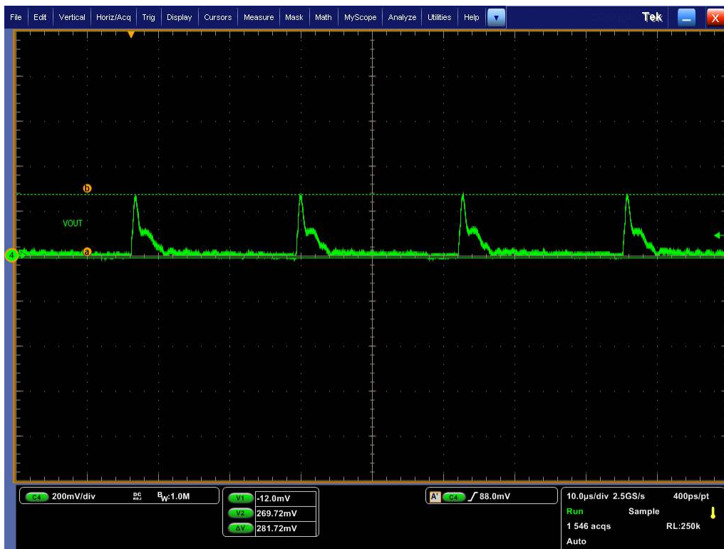
Figure 5-16. Output Voltage Ripple: VIN = 50 V, Load = 1.3 A
