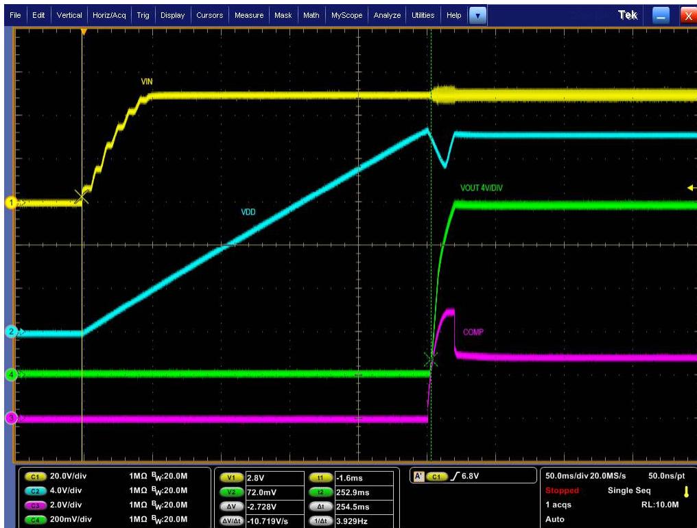
Figure 5-8. Start-Up 2: VIN = 50 V, Load = 1.3 A
