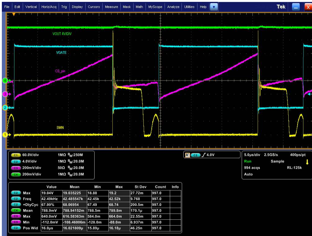
Figure 5-20. Steady State: VIN = 50 V, Load = 1.3 A
