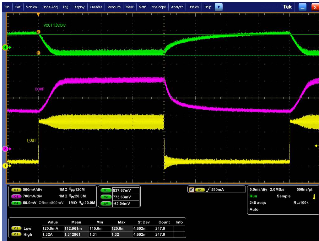
Figure 5-24. Transient Response: VIN = 50 V, Load = 100 mA to 1.3 A at 25 Hz, 50% duty
