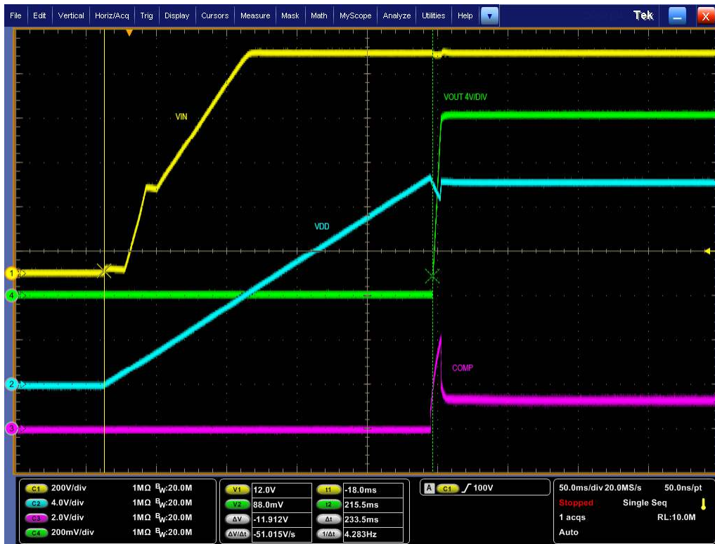
Figure 5-9. Start-Up 3: VIN = 1000 V, Load = 0.25 A
