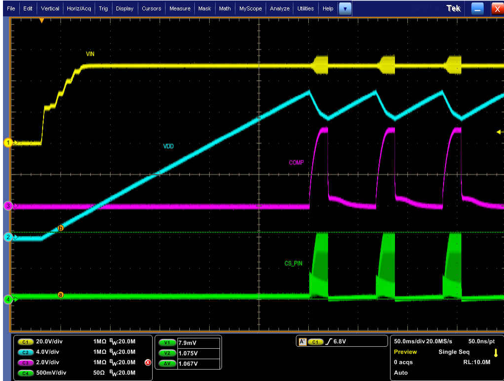
Figure 5-27. 50 VIN, Startup with output shorted to ground
