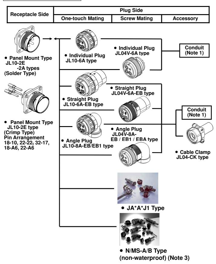
Note 1) Please contact us or conduit manufacturer for detailed use of a conduit. Note 2) Please refer to individual catalogs for consideration of JL04V Series, N/MS-A/B Series, and J1 type JA\*A Series.
