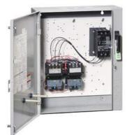
2-speed 3-phase motor starter Size 0 Two separate windings Constant or variable torque Solid-state overload relays Low SPD OLR range 0.75-3.4A High SPD OLR range 3-12A 110V 50HZ / 120V 60HZ coil Combination type 10Amp circuit breaker Enclosure NEMA type 4/12 Water/dust tight for outdoors
