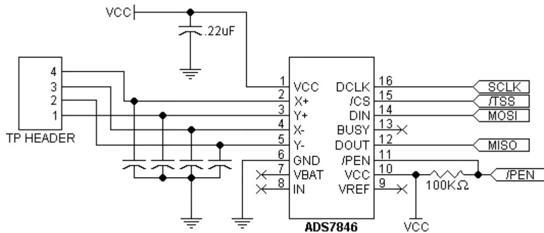
The 4 noise filtering capacitors between the TP HEADER and Burr-Brown device may or may not be needed, but it is recommended you design them in because you can always leave them unpopulated. Whether or not you need the noise filtering capacitors will depend on the size of the touch panel, as well as the environment in which the product will be used. For applications requiring the use of the noise filtering capacitors, .01uF (+/- 10%) capacitors will normally address the problem.
