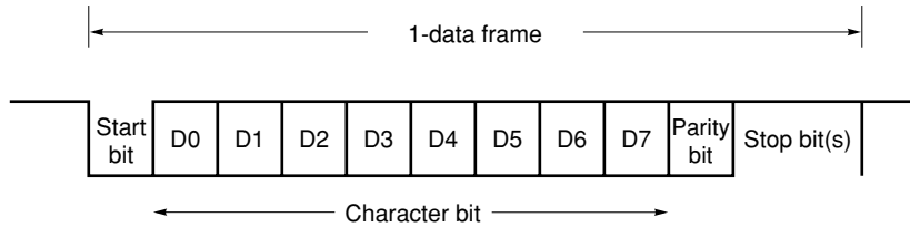
Figure 17-7. Asynchronous Serial Interface Transmit/Receive Data Format
