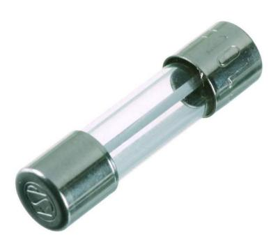
Fuse, Dimensions: 5x20 mm, Trigger characteristic: Fast-acting (F); Rated voltage: 250 V, Rated current: 0.8 A
