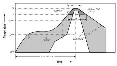
Ramp-up rate = 3 °C/sec. max. Ramp-down rate = 6 °C/sec. max.  $T_L = 217$  °C  $t_L = 60-150$  sec.
