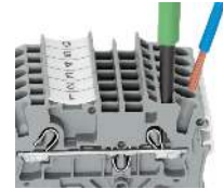
Inserting a conductor via operating tool: Connecting fine-stranded conductors without ferrules, or small cross-sectional conductors that cannot be pushed in, is performed similarly to the original CAGE CLAMP® – just use an operating tool. Advantage: To open the clamp, the operating tool is inserted vertically. The conductor entry is less than 15 degrees for easier wiring.
