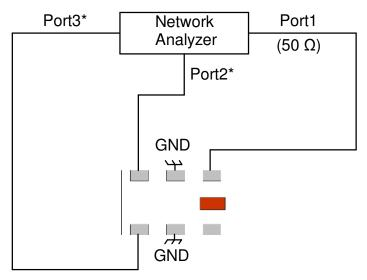
\*Impedance for ports 2 and 3=1/2(Balanced impedance)
