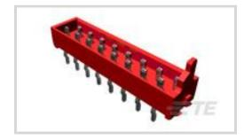
Connector System: Board-to-Board Number of Positions: 6 Centerline (Pitch): 1.27 mm [.05 in ] PCB Mount Retention: With PCB Mount Retention Type: Kinked Solder Tails All Male-on-Board Connector, Micro-MaTch (36)
