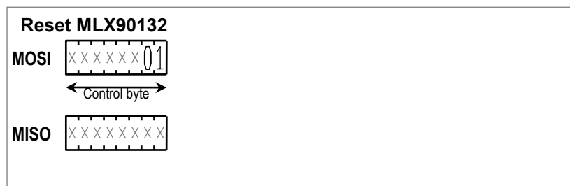
Figure 9: SPI communication reset the MLX90132
